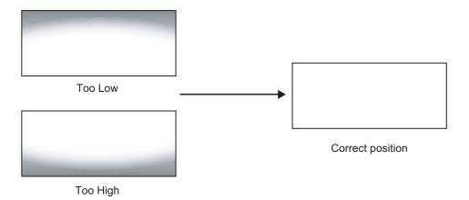
4. When the height is properly set, tighten the Pitch/Y-Adjustment Screws to secure the lens in place.
